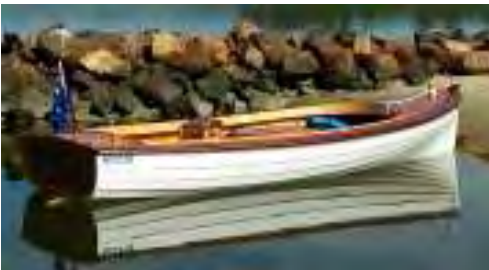
LILLIAN ROSE is a classic design traditionally built clinker launch. Marine ply hull with celery top steam bent ribs and red cedar and silver ash deck. She has a 21hp Nanni diesel and wheel steering. Built by Scott with assistance from family. Scott Garven
