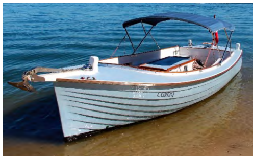
SALTY DOG Built in 1971 and Fully restored by Doug Fielding, Regatta Marine in 2010 Carvel clinker, maple planking and spotted gum ribs. Powered by Holden 202 Doug Fielding
