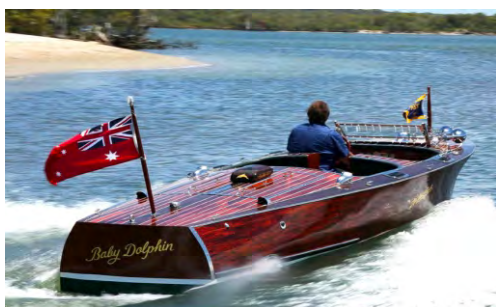
BABY DOLPHIN A 1928 Hacker Craft replica, American speed boat powered by a 500 cubic inch Cadillac motor. She is a 22-footer and I have been enjoying her for 6 years now. I built her from Brazilian Mahogany & finished her in 2013. I put her together from station frames drawn on a large piece of brown paper & a hand full of photos sent to me from the company in Lake George upstate New York. Geoffrey Tyler
